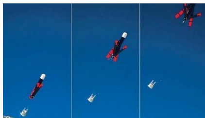
Figure 2: After the flight of the UAV, the tail and wings open
