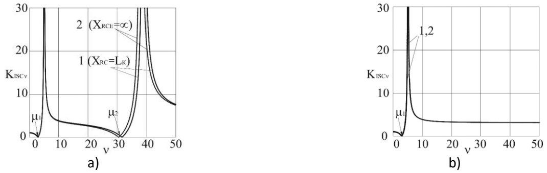
Figure 7: Current harmonics reduction coefficients frequency characteristics K_{IIIv} : a) for APLC2; b) for APLC3
