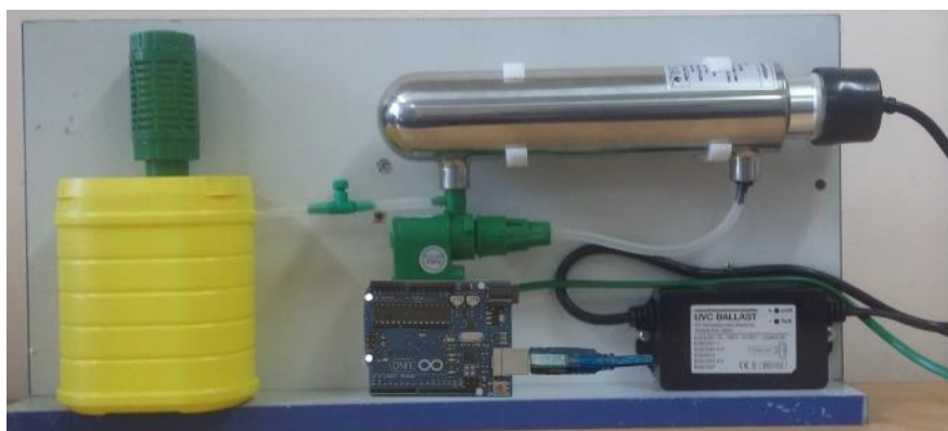
Figure 3: General view of a laboratory bench for collecting and analyzing gases
